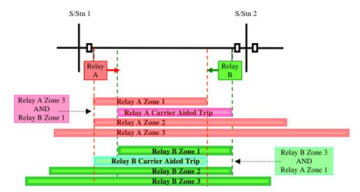
The relay is arranged to send a signal when its Zone 1 picks up.
