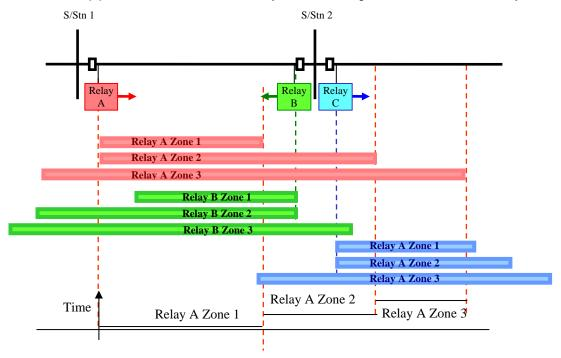
The disadvantage of such a scheme is that faults in the last 20% of the line are cleared after the Zone 2 time delay. This may be acceptable for lower voltage distribution systems, but for important circuits or higher voltage systems additional schemes are available to improve the tripping of the relay.
